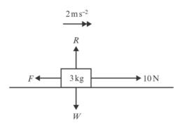
Resultant force = ma  $m = 3 \text{ kg}, a = 2 \text{ ms}^{-2}$   $R (\rightarrow), 10 - F = 3 \times 2 = 6$  F = 10 - 6The force due to friction is 4 N.
