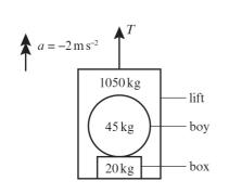
**a** F = maTaking up as positive:  $(1050 + 45 + 20) \times -2 = T - (1050 + 45 + 20)g$ T = 1115(g - 2) $T = 1115 \times 7.8$ The tension in the cable is 8697 N.
